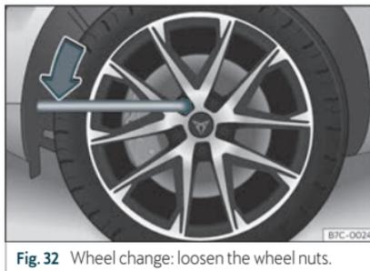
**Fig. 32** Wheel change: loosen the wheel nuts.
