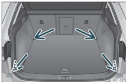
Fig. 110 In the luggage compartment: fastening rings.
