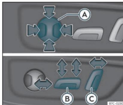
Fig. 97 Driver's seat: electric seat settings.
