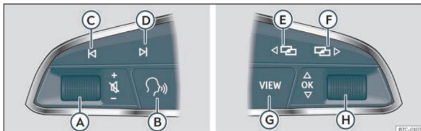
Fig. 65 Controls on the steering wheel.
