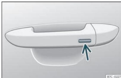
Fig. 86 Door handle: sensor surface.
