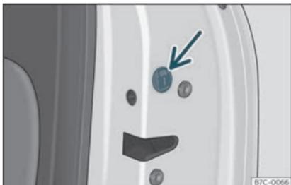
Fig. 75 Locking the door manually.
