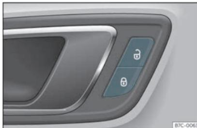
Fig. 70 Driver's door: central locking switch.
