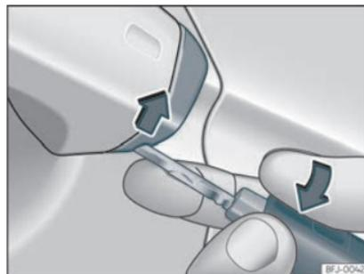
**Fig. 74** Driver door handle: lever the cover off
