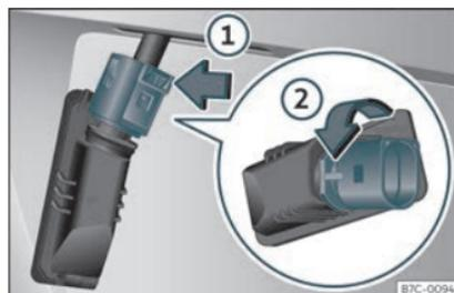
**Fig. 52** number plate light: remove the bulb holder.
