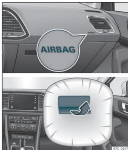
Fig. 13 Front passenger airbag located in dash panel.
