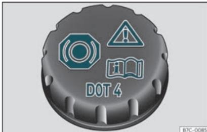
**Fig. 261** Engine compartment: brake fluid reservoir cap.
