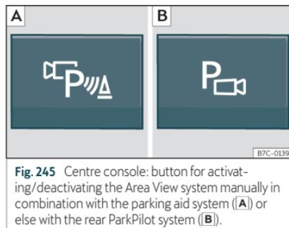
**Fig. 245** Centre console: button for activating/deactivating the Area View system manually in combination with the parking aid system (A) or else with the rear ParkPilot system (B).
