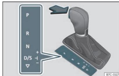
**Fig. 200** Selector lever lock.
