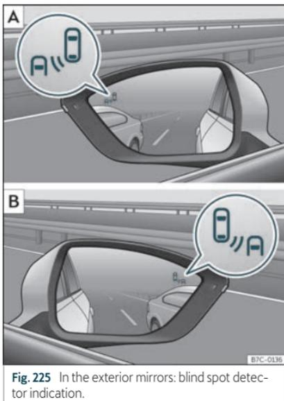
**Fig. 225** In the exterior mirrors: blind spot detector indication.
