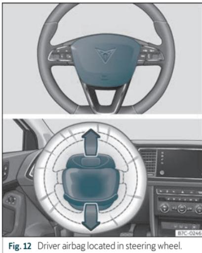
Fig. 12 Driver airbag located in steering wheel.
