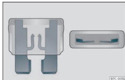
**Fig. 46** Image of a blown fuse.
