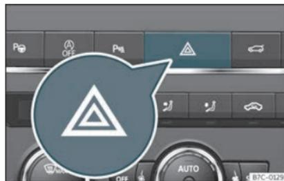
Fig. 90 Dash panel: hazard warning lights switch
