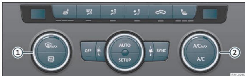
Fig. 122 In the centre console: Climatronic controls.
