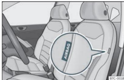
**Fig. 18** Side airbag in driver's seat.
