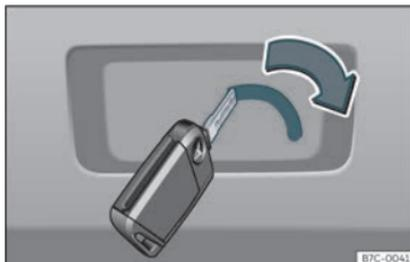
**Fig. 82** Detail of the luggage compartment: emergency unlocking
