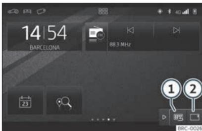
**Fig. 140** Other MirrorLink function buttons.
