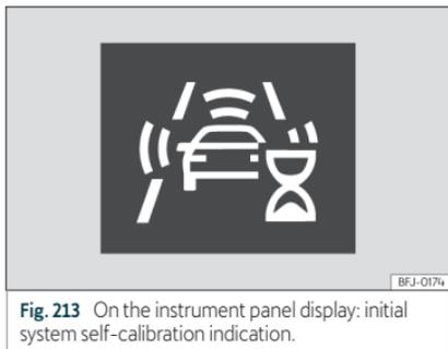
**Fig. 213** On the instrument panel display: initial system self-calibration indication.
