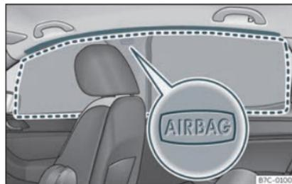
**Fig. 20** Location of head-protection airbags.
