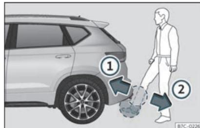
Fig. 80 Rear lid with sensor-controlled opening (Easy Open).
