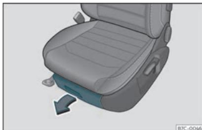
**Fig. 118** Storage compartment under the front seats.
