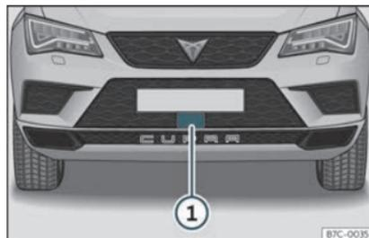
**Fig. 216** On the front bumper: radar sensors.
