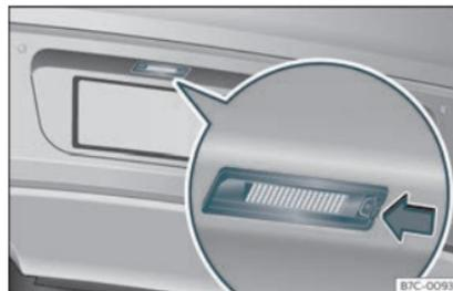
**Fig. 51** In the rear bumper: Number plate light.
