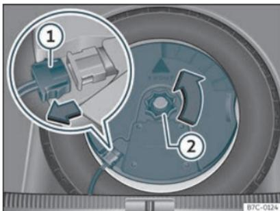
**Fig. 268** In the luggage compartment: remove the subwoofer.
