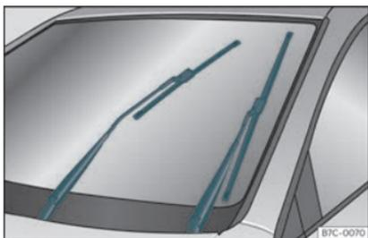
Fig. 35 Wipers in service position.
