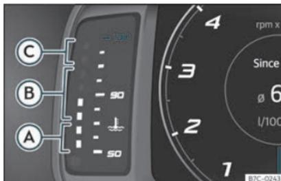
Fig. 60 Engine coolant temperature indicator.
