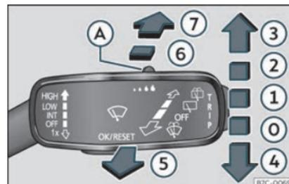
**Fig. 91** Operating the windscreen wiper and rear wiper.
