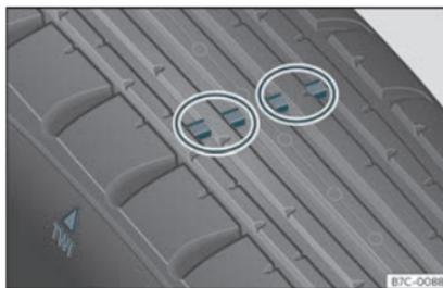
Fig. 264 Tyre profile: tread wear indicators.
