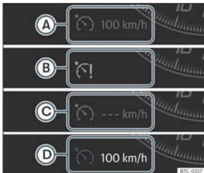
**Fig. 205** Instrument panel display: GRA status indications.
