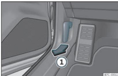
Fig. 254 Release lever in the driver's footwell area.
