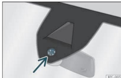
**Fig. 124** Windscreen humidity and temperature sensor.
