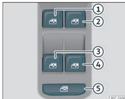
**Fig. 83** Detail of the driver's door: window controls.
