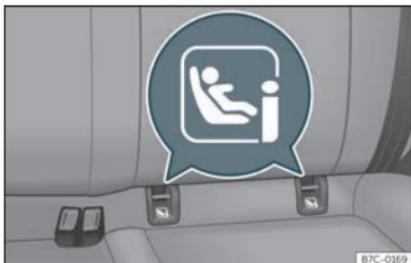
**Fig. 24** Rear seat: ISOFIX/i-Size securing rings.
